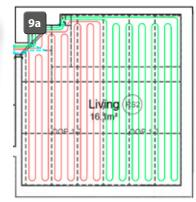
9. Before laying pipe make sure all pipe channels are clear from debris, check and familiarise yourself with the pipe layout drawing (9a) plan where to begin and the pipe routes for each individual loop of pipe.
