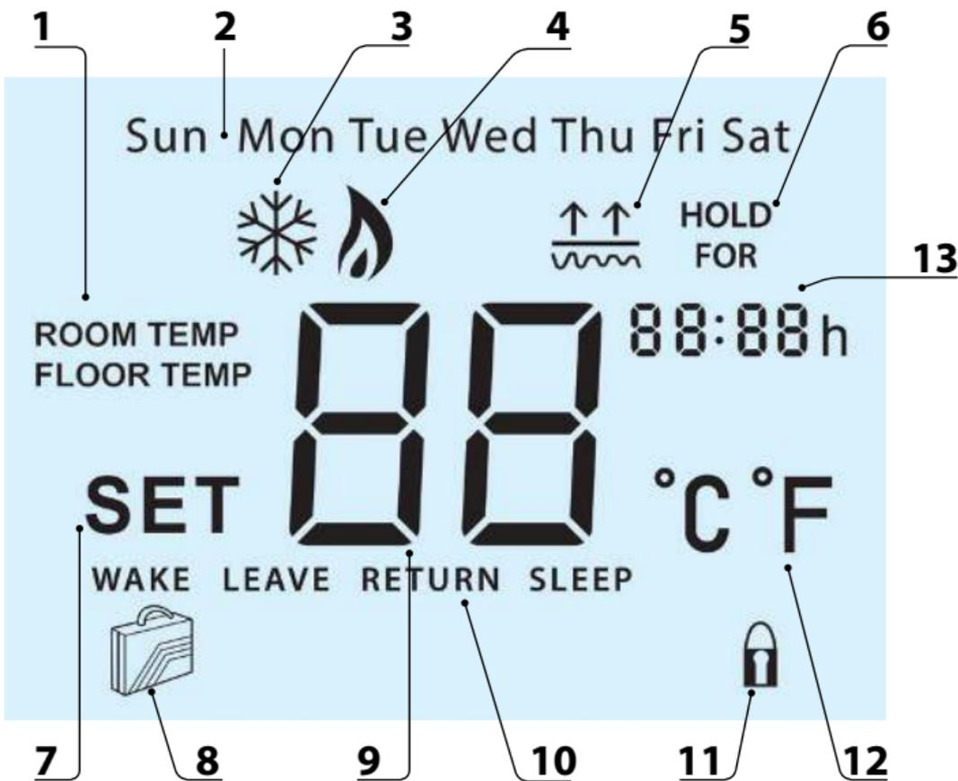
1. Room/Floor Temp - Indicates the current temperature sensor mode.
