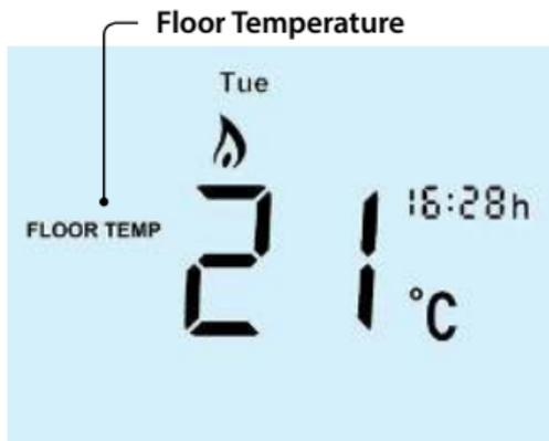
*Note: Built in air sensor only MUST NOT be used to control electric underfloor heating. Floor sensor only or built in air & floor sensor together must be used.*
