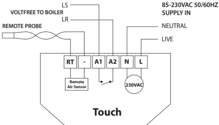
LS & LR ARE NORMALLY THE ROOM THERMOSTAT CONNECTIONS
