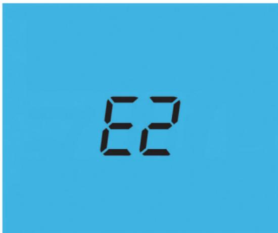
Check the sensor is correctly connected to the RT1 and - terminals at the rear of the thermostat (see wiring diagrams on page 26-28).
