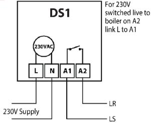
LS & LR ARE NORMALLY THE ROOM THERMOSTAT CONNECTIONS
