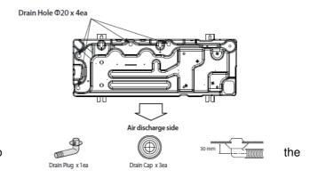
The unit must have adequate drainage away from the unit; it can produce up to  $6\,L$  / hour. There is a drainage kit included which we recommend you don't use, its best to let the unit drain into the ground. If a drip tray is used it must be 25mm longer and wider than the base of the unit to catch all the drips.
