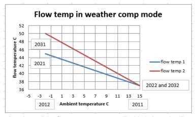
You will see 0.0C on the screen; the unit is using weather compensation function to work out the water temperature. If you need to boost the heating water temp this can be done by pressing the silver up and down buttons. This boosts the radiators by up to +5 C but warning this will cost more money to run.
