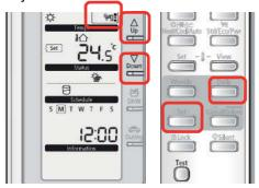
Press daily button once, no 1 and on shows, press grey set, press up or down until the tap symbol shows at the top of the screen with 2 dots press grey set, adjust hours with up or down button to 3 am press grey set, minutes flash press set. Now everything flashes press set (grey). No 2 appears do the same again but for 15-00.
