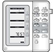
The controller will display TEST. Immediately press the top left button to turn the pump on and leave it running while in test mode to avoid a fault.
