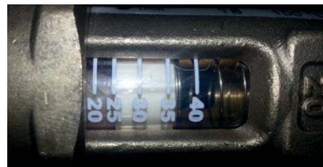
**If the flow rate is too low you need to fix this before moving on.**
