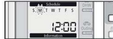
The hours will flash adjust this with the silver up and down buttons, press grey set.
