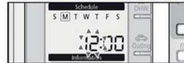
The minutes will flash, adjust this with the silver up and down buttons, press grey set you are back to the normal screen.
