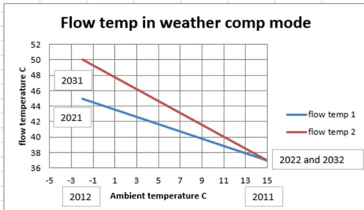
**You will see 0.0C on the screen;** the unit is using weather compensation function to work out the water temperature. If you need to boost the heating water temp this can be done by pressing the silver up and down buttons. This boosts the radiators by up to +5 C but warning this will cost more money to run.
