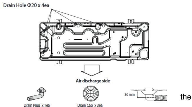
The unit must have adequate drainage away from the unit; it can produce up to 6 L / hour.
