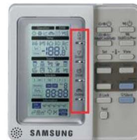
You should see 0.0C on the screen this means the unit is under external control from a room thermostat.
