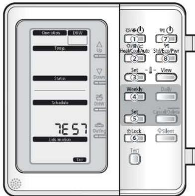
The controller will display TEST. Immediately press the top left button to turn the pump on and leave it running while in test mode to avoid a fault.
