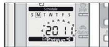
To adjust this setting press **set** again the setting will appear at the top of the screen, adjust it with the silver up down buttons and press **set** again, scroll up to the next field setting using the up and down buttons and repeat.
