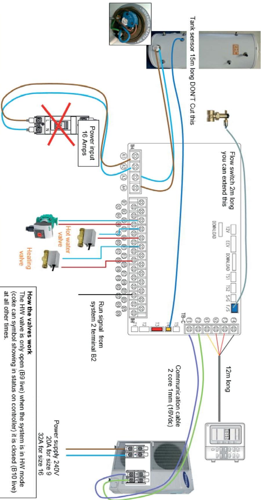
**BOTH** heat pump control boxes **MUST** be powered from a single RCD or RCBO and the internal breakers removed, wire the power straight into A1 and A2 of the PCB
