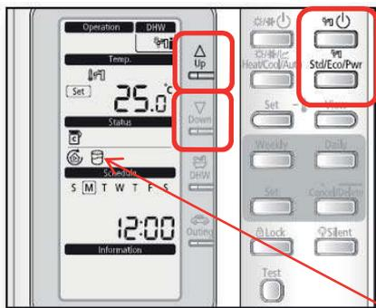
Press Hot water on off button to start the unit, top right button.
