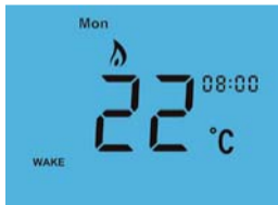
For 7 Day programming, only Mon is displayed in the day indicator field.
