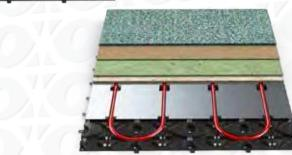
The Profix™ Panel, when combined with the Profix™ Plate, provides a very quick and easy to install ultra-low profile solution for use with warm water underfloor heating systems incorporating either a 10mm or 12mm pipe.
