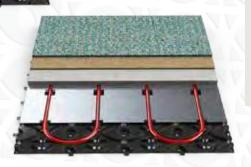
The high structural integrity of the Profix™ Panel enables the direct application of a highly thermally conductive screed replacement board which, in addition to optimising heat transfer, enables either a tiled, vinyl, or thin laminate floor to be bonded directly to it or for a low tog carpet and underlay to be laid directly onto it.
