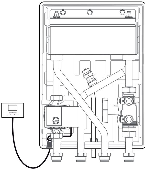
The external wiring to be grounded. The polarity must be correct and consistent with the standards.
