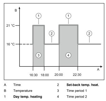
You can specify the temperatures (**Day temp. heating** and **Set-back temp. heat.**) in the Setting the **Desired temperatures** ( $\rightarrow$  Page 10) function.
