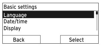
Turn the rotary knob until the list entry **Display** is highlighted.
