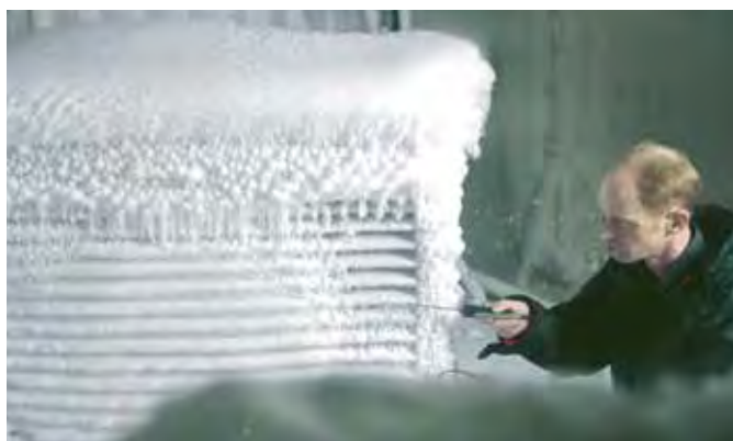
Testing teams operate the units in extreme climatic conditions in the cold chamber.
