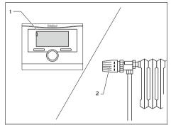
Set the room thermostat or the weather compensator (1) and thermostatic radiator valves (2) as specified in the relevant instructions for these accessories.
