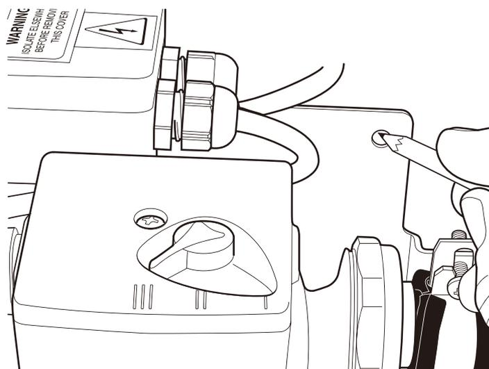
Remove the unit and drill (8mm masonry drill) and plug the holes. Align and secure the unit to the wall with the screws provided. The unit is now ready for connecting to the primary heating supply and underfloor heating loops. If appropriate the unit can be connected to the underfloor heating loop(s), filled and pressurised via the integral ball valves and then locked off for floor screeding before making the boiler connection.
