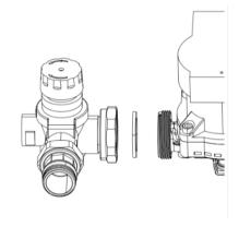
1.2 Install the gasket into the connecting nut of the water supply system component, and then match the connecting nut with the external thread of the water pump and tighten it. Ensure that water supply system components, gaskets and pumps are in sealed fit.
